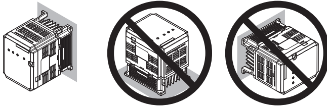
Figure 8 Correct Installation Orientation (Braking Unit)
